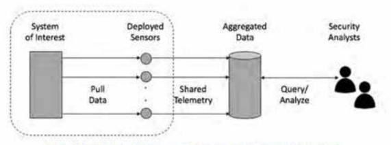
Figure 3-1. Traditional Telemetry Collection and Aggregation Method
